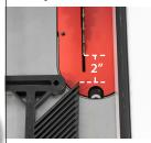
Always make sure that the last finger on the featherboard is at least 2" in FRONT of the blade or cutter on the in-feed side. This ensures that the stock will not "pinch" against the blade or cutter when feeding your stock through.
